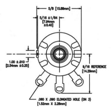
A & B & C DIMENSIONAL VARIABLE. TOLERANCES NOT SPECIFIED ± 1/32 [0.80mm]
